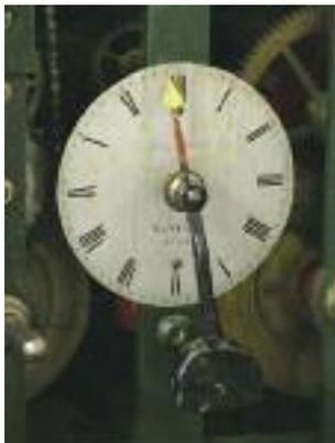
The clock still had to be adjusted by hand to and from British Summer Time until September 2018 when an auto-regulator was installed. This was a radio signalled solenoid switch to the pendulum, which acted as an automatic timer and enabled the clock to switch automatically from Greenwich Mean Time to British Summer Time. This installation was paid for by a bequest from John Plaister, a member of the Christ Church congregation, Trustee of the Friends and expert horologist.
